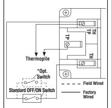
\* Optional Kits Installed - OFF/ON wall switch, wall thermostat or remote control receiver. Note: Turn the appliance-mounted OFF/ON burner control switch to the OFF position if any of these kits are installed.
